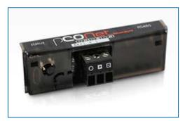
Connect the serial card to your laptop by using the RS485 to USB converter.
