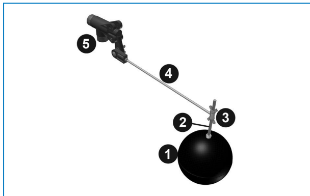
Water make-up valve assembly
