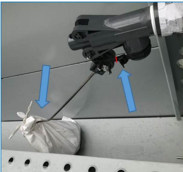
Fixation and wrapping of float ball
